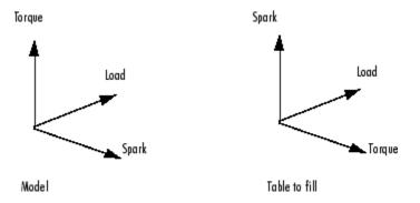
In the diagram of a table shown, the *x*- and *y*-axes represent the normalizers (which you want to be spark and load) and the *z*-axis is the output at each breakpoint (torque). To fill this table correctly from the model is a two-step process. First you need to fill a table that has the same input and output as the model, and then fill a second table by inversion.
